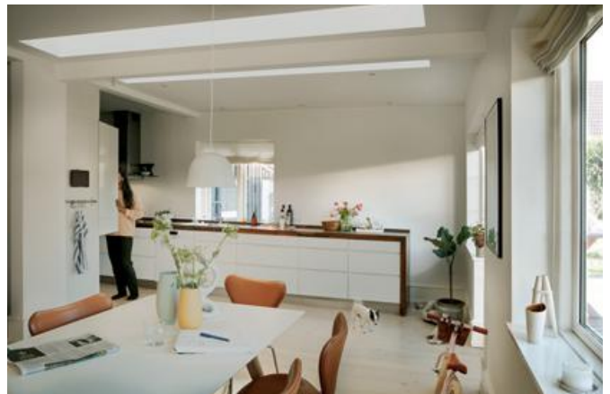
Double layer glazing with Sun coating (Sun) and with a light transmittance of 61%.
